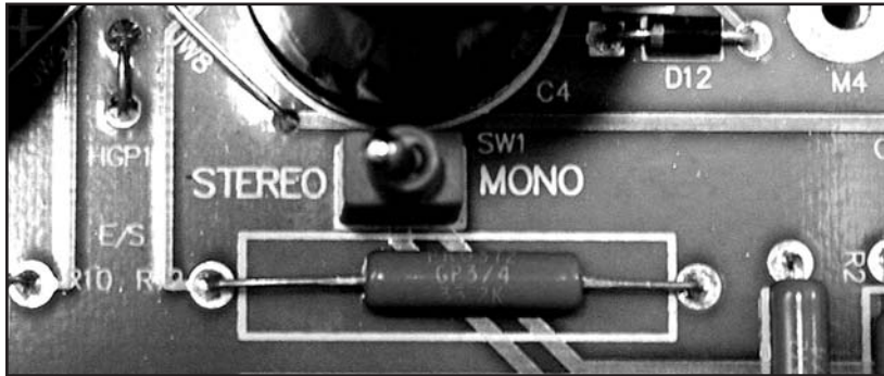
Setting the internal switch to mono converts the 100 watt per channel stereo amplifier into a 350-watt monophonic amplifier. As such, it will have tremendous speaker control with powerful dynamics.
